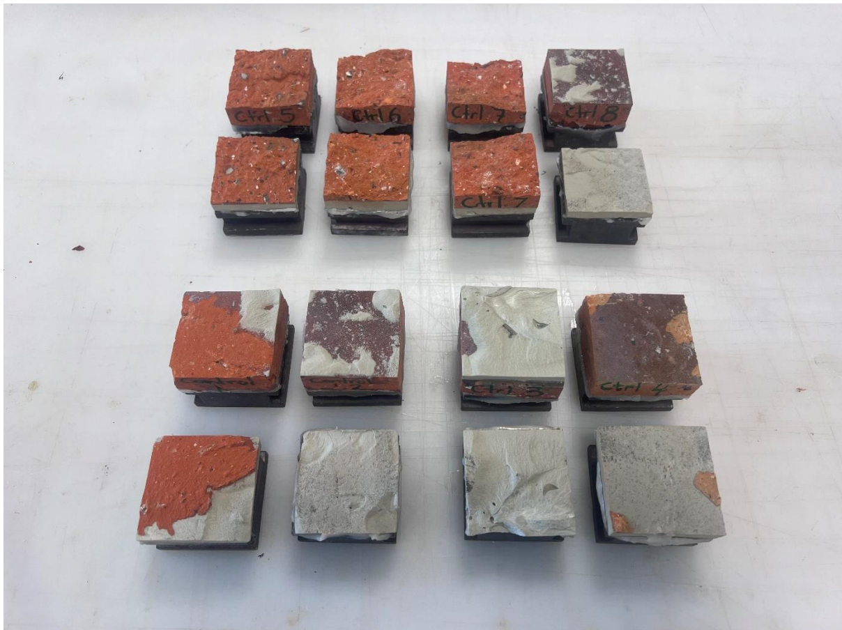
Figure 2. Images of the tested control samples showing the failure mode. Samples 1-4 bottom row (left to right), samples 5-8 top row (left to right)
